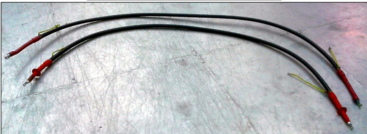
Fig. 67 Prepared cable samples for accelerated aging tests
