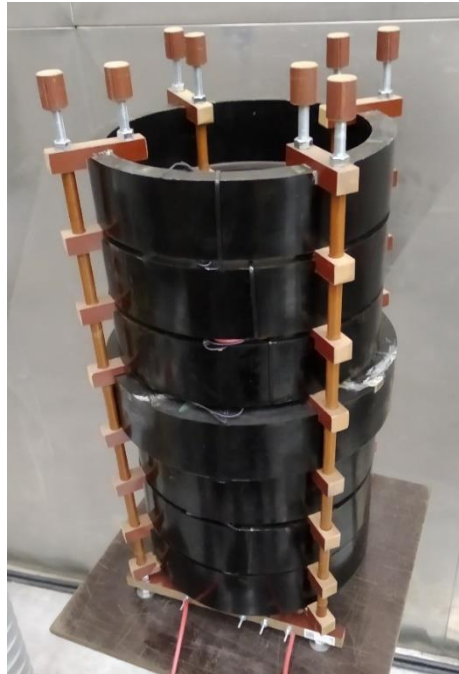
Air-core inductor TRONIC 11.7 H, 15 kV, 1 A
