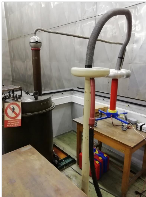
Fig. 73 Setup of partial discharge measurements
